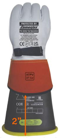
The minimum distance from the leather protector cuff to the bead of the rubber glove for this Class 2 glove is 2 inches.
