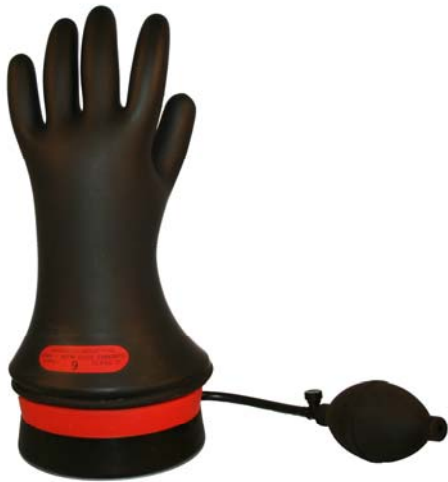
The IG0-11-9 (Class 0, 11" length glove, size 9) with the Cementex glove inflator (CPGI), which enables thorough visual inspections which are required prior to each use.
